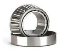
PFI Taper Roller Bearings take higher radial loads and axial loads due to special heat treated steel. PFI Taper Roller Bearings are also available in two row versions for Front & Rear Wheel HUB Bearing units to support axial loads in either direction. Optimized designs can be supplied with high strength cages for arduous applications and sealed with triple lip sealing innovations to maintain long life.
