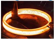
All PFI bearings are manufactured from forged long life steel with heat treatment Bearings in Automotive Wheel applications with ability to take exceptionally hi-impact loads. This results in outstanding durability and long life. PFI specially hardened case Raceways with a forged durable core increases higher load carrying ability on Australian tough roads.
